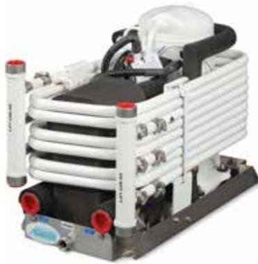
Marine Air MCGXLP Titan modular chillers use titanium condensers to greatly increase durability and product lifespan. Titanium is unaffected by the punishing combination of saltwater, invasive marine life, and the harsh acids used for routine cleaning of the condenser coil. Titan service life is greatly extended compared to cupronickel systems—the industry standard—which inevitably suffer catastrophic failure from corrosion and erosion in the harsh marine environment.
