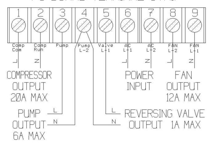
"L" AND "N" REPRESENT "LINE" AND "NEUTRAL" FOR A 115V SYSTEM "L" AND "N" WOULD BE "LI" AND "L2" FOR A 23ØV SYSTEM
