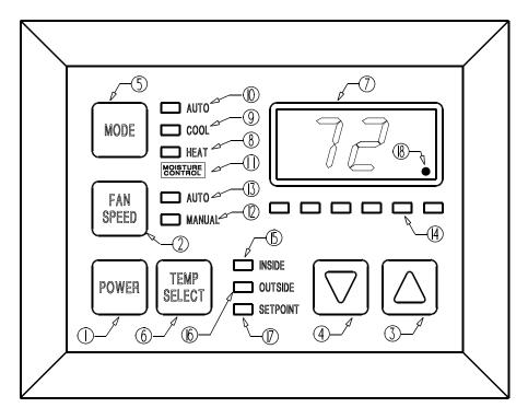
Figure 1: Tempwise 2001 Control Buttons and Indicator Displays
