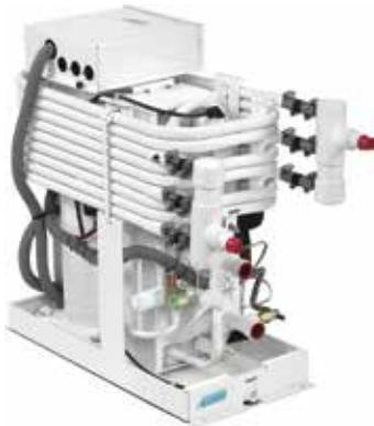
Marine Air MCGX Titan modular chillers use titanium condensers to greatly increase durability and product lifespan. Titanium is unaffected by the punishing combination of saltwater, invasive marine life, and the harsh acids used for routine cleaning of the condenser coil. Titan service life is greatly extended compared to cupronickel systems—the industry standard—which inevitably suffer catastrophic failure from corrosion and erosion in the harsh marine environment.
