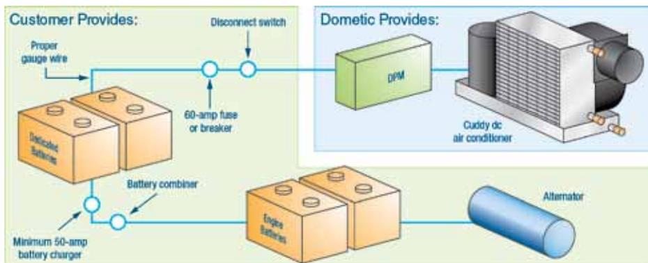
The customer must provide the right type of batteries and the right type of battery charger. Use only deep-cycle AGM or gel-cell batteries, do not use wet-cell batteries. The battery charger must be rated for the type of battery you use. The Cuddy dc required a dedicated battery bank. To maximize runtime, we recommend using at least two batteries in the bank. The more cells, the longer the runtime. All batteries used must be of the same type - all AGM or all gel-cel - and the same age.
