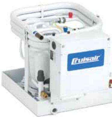
R Type remote condensing units are the next generation of seawater-cooled, reverse-cycle heat pumps for cooling and heating in marine applications. Small R Type units are available in capacities from 5,000 to 16,000 BTU/hr.
