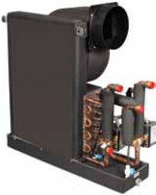
The ATV is a chilled water air handler designed for applications where very little depth is available. In the "4-pipe" configuration there are two separate sets of valves and heat exchangers for cooling and for heating. Two pipes connect to the chiller system to provide cooling, and two pipes connect to an auxiliary heat source, such as a boiler, to provide heating.
