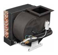
Marine Air's EFD 24,000 BTU/hr evaporator for split-system air conditioning features a compact, modular design. For maximum efficiency, the plenum chambers are increased and the coil has enhanced fins and rifled tubing. This unit also offers easy disassembly for access to components for maintenance. It works with Marine Air R-22 or R-417A condensers.
