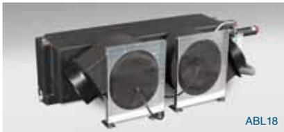
Due to the upright blower orientation, ABL models are taller than ATL models, but not as deep. ABL air handlers can be suspended from above or supported from beneath. Vibration-isolation mounts are sold separately.
