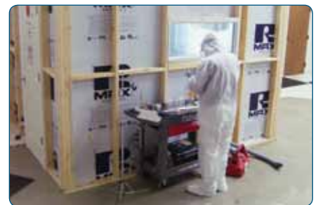
Exterior of the Breathe Easy Air Purifier test chamber at Environmental Diagnostics Laboratory
